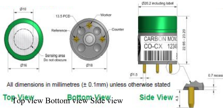
Figure 1 Schematic Diagram of CO-CX
