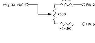
Figure 2 Power Supply Circuit of Sensing Bridge
