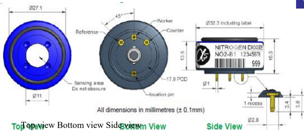
Figure 1 schematic diagram of NO2-B1
